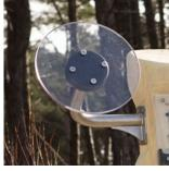
Rotary elements made of polycarbonate,
