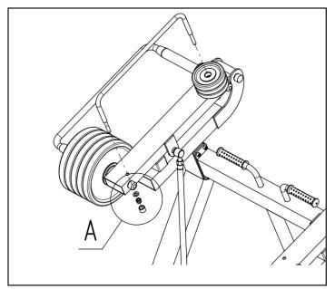
On both sides of the exercise machine: place weight plates (3 pcs of 2,5 kg each), as shown in the figure. Then attach a small guide rail to a lever by nuts. It's done!
