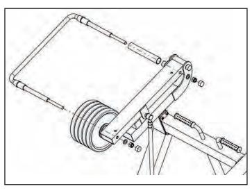
On both sides of the exercise machine: insert the guide rail into the sleeve. Fasten the ends by nuts.
