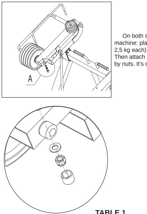
On both sides of the exercise machine: place weight plates (3 pcs of 2,5 kg each), as shown in the figure. Then attach a small guide rail to a lever by nuts. It's done!
