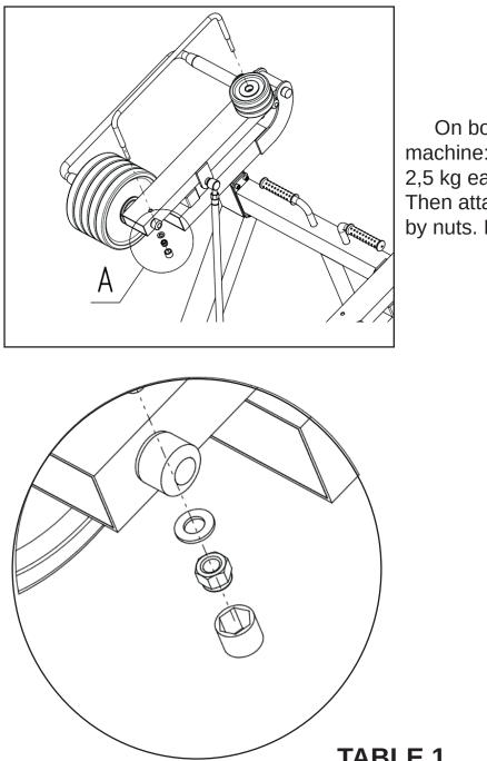
On both sides of the exercise machine: place weight plates (3 pcs of 2,5 kg each), as shown in the figure. Then attach a small guide rail to a lever by nuts. It's done!
